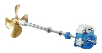
The Switch PMM can be used as a direct-drive propulsion motor, either conventionally with its own bearings and shaft or as a novel concept, utilizing the common bearings between the propulsion shaft and motor. A tandem configuration is also possible on request.
