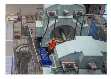
Complete full-power testing with machines and drives up to 18 MW is available at our Large Drive Test Center in Lappeenranta, Finland.
