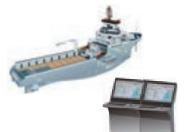
The DPS is a system that maintains the vessel's position and heading at a constant level using only the vessel's onboard propulsion system. It efficiently controls the propulsion system against disturbances such as wind and tidal waves and keeps the ship at a fixed point while saving energy.
